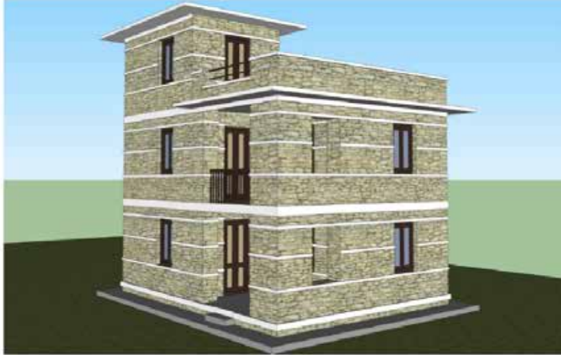
Model SMC-2.6: STONE MASONRY IN CEMENT MORTAR
