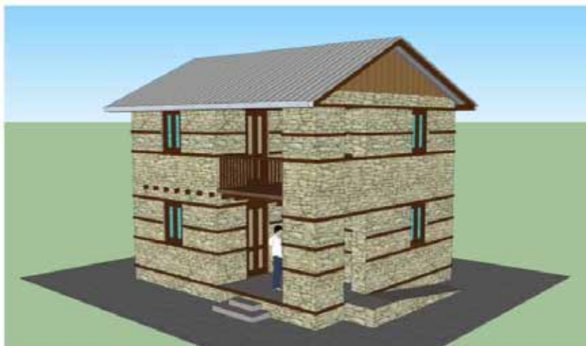
Model SMC-2.2: STONE MASONRY IN CEMENT MORTAR
